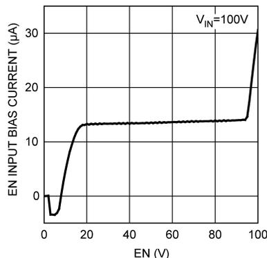
Figure 28. EN Bias Current vs Voltage
