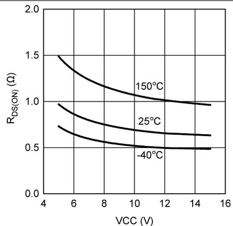
Figure 9. LO Low R<sub>DS(ON)</sub> vs VCC
