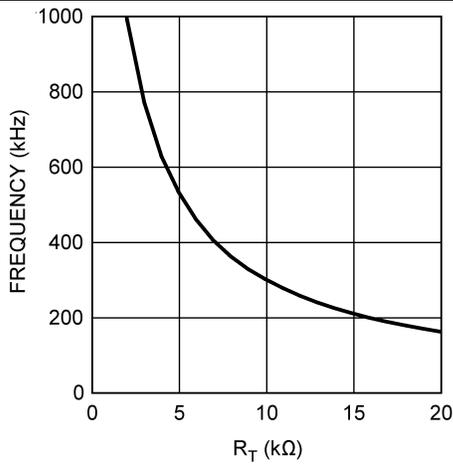
Figure 13. Frequency vs  $R_T$
