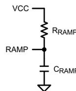
**Figure 38.  $R_{RAMP}$  to VCC for  $V_{OUT} > 7.5\text{ V}$**
