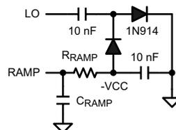
**Figure 39.  $R_{RAMP}$  to -VCC for  $V_{OUT} < 7.5\text{ V}$**
