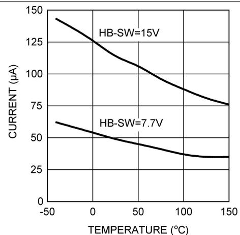
Figure 12. HB DC Bias Current vs Temperature
