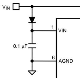
Figure 26. Input Blocking Diode for VCCX > VIN
