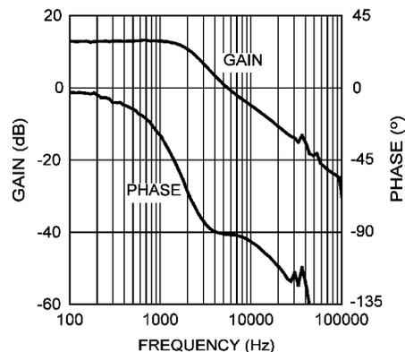
**Figure 35. Modulator Gain and Phase**
