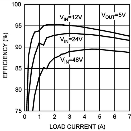
Figure 40. Efficiency With 6- $\mu$ H Copper Inductor
