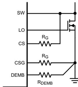
**Figure 30.  $R_{DS(ON)}$  Current Sensing without Diode Emulation**
