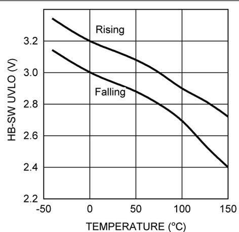
Figure 10. HB to SW UVLO vs Temperature
