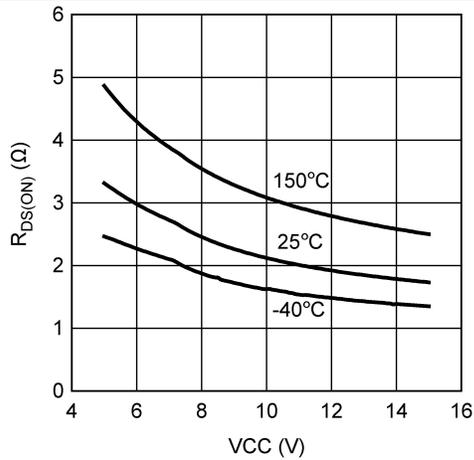
Figure 7. LO High R<sub>DS(ON)</sub> vs VCC
