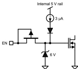
Figure 27. Enable Circuit
