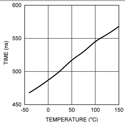
Figure 11. Forced HO Off-time vs Temperature VCCX = 5 V
