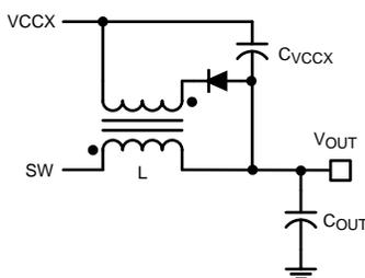
Figure 25. VCCX Bias Supply with Additional Inductor Winding
