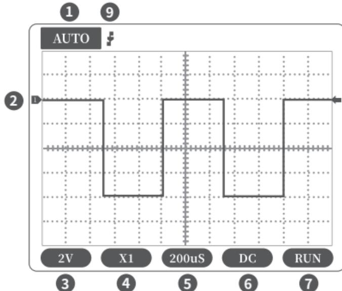
①Trigger mode indicator icon, Auto means automatic trigger, Single means single trigger, Normal means normal trigger.
