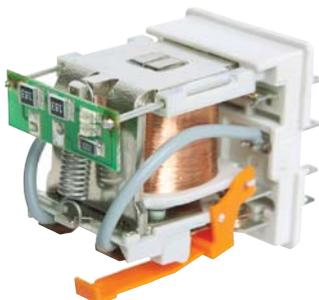
**Application of electronics made in the SMD technology:** additional equipment L (LED diode) and D (diode) are located on the printed circuit board; the change of the position of the LED diode and optimization of the quality and intensity of its light provide certainty that the relay is in operation status when the LED is on.
