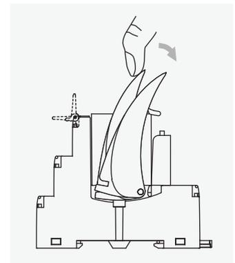
Removing the relay from the socket
