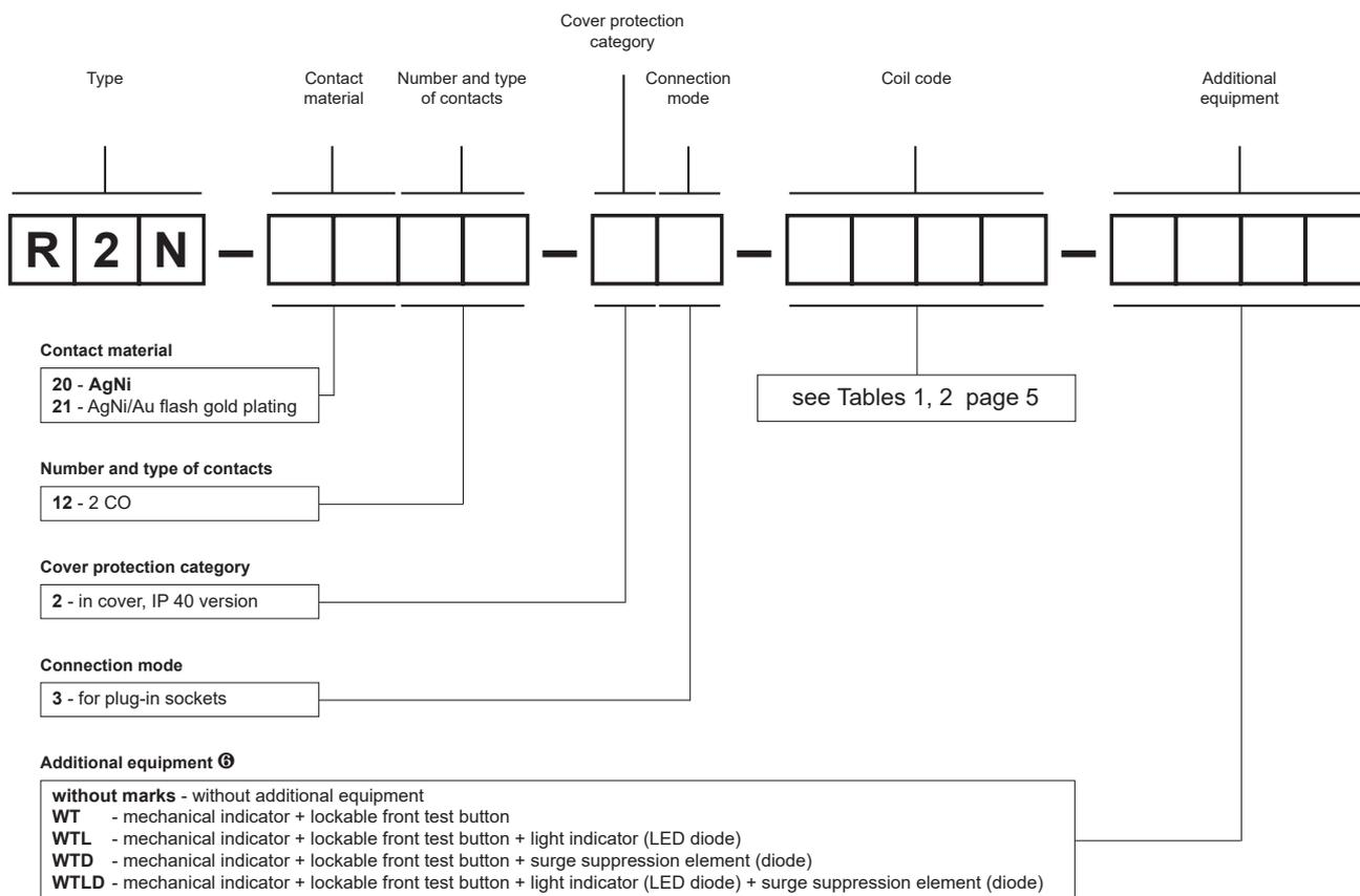
Ⓜ T - orange colour (AC coils), green (DC coils). WT - standard equipment of relays. WTD, WTLD - available only in relays with DC coils.
