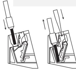
The drawings present inserting wire into the Push-in terminal and removing wire using the button releasing a clamp (assembly without tools).
