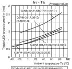
Io=Continuous Load Current Ratings, t<1s G3VM-61B1/61E1/351B/351E/401B/401E G3VM-91B1/91E1/391B351E/401B21 ID=Continuous Load Current Ratings, t<1s, Connection A G3VM-353A/353D: IoFF=10µA, G3VM-353B/353E: IoFF=10µA, Connection A
