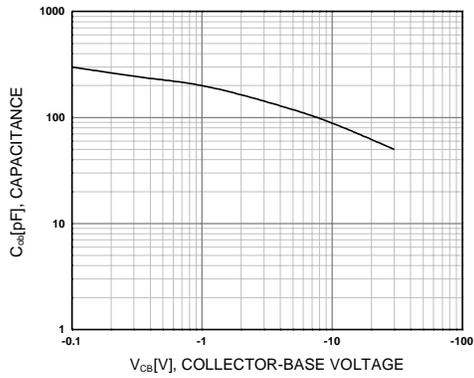
Figure 3. Collector Capacitance
