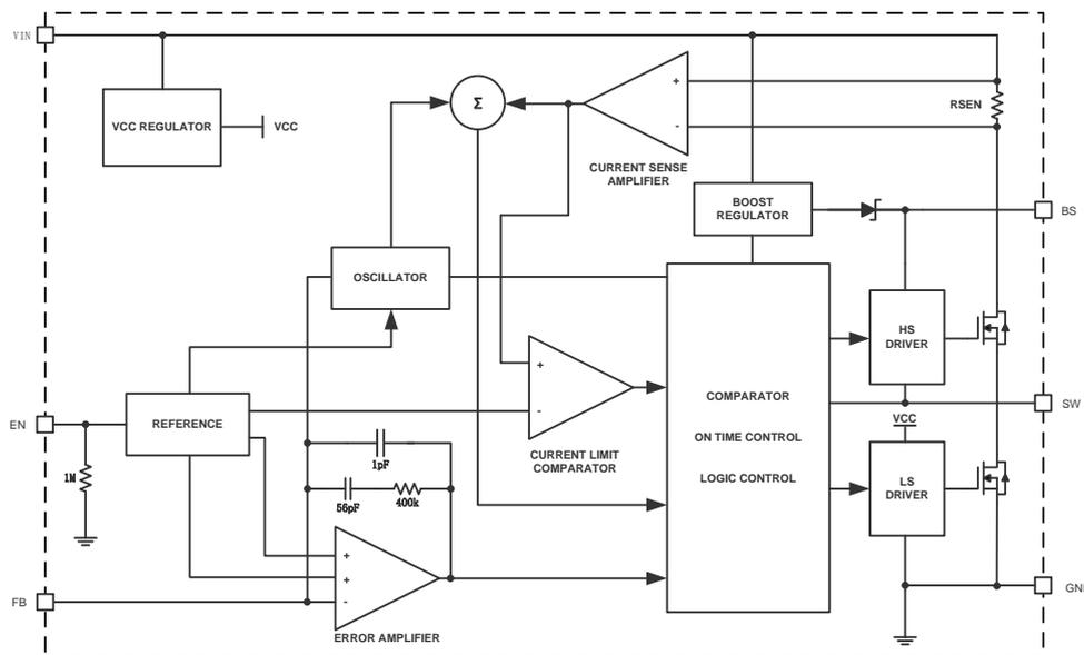
Figure 2. RY3834 Block Diagram
